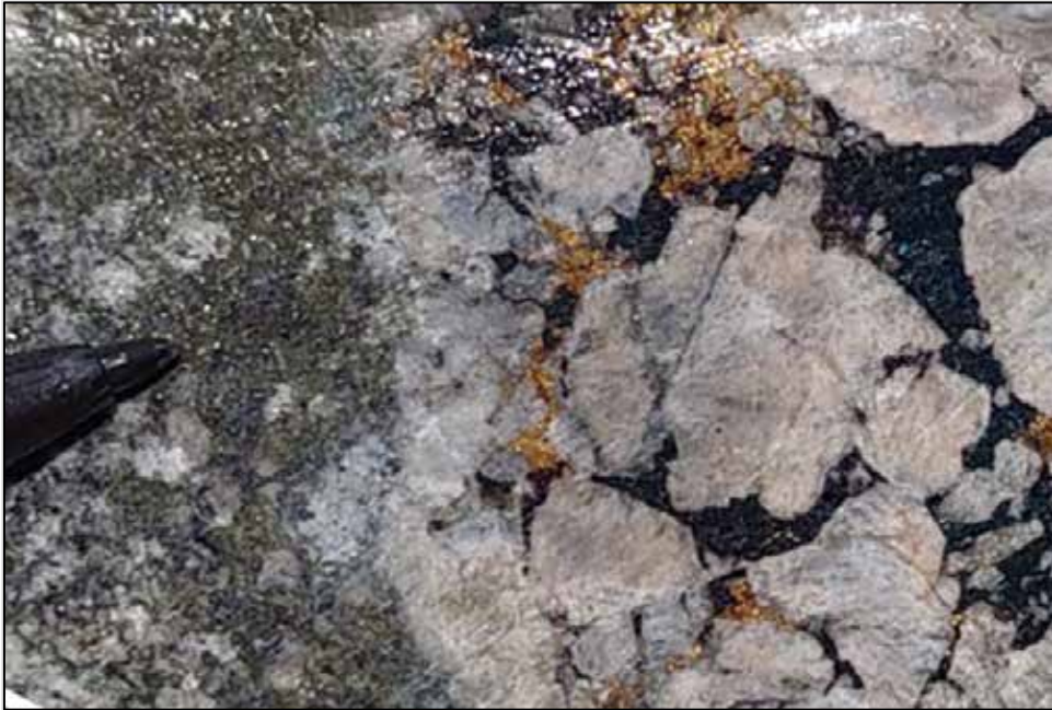
Photo 6-4: Balut Dyke- Mafic facies in contact with hydrothermal breccia with Felsic Balut cemented by bornite and chalcopyrite.
