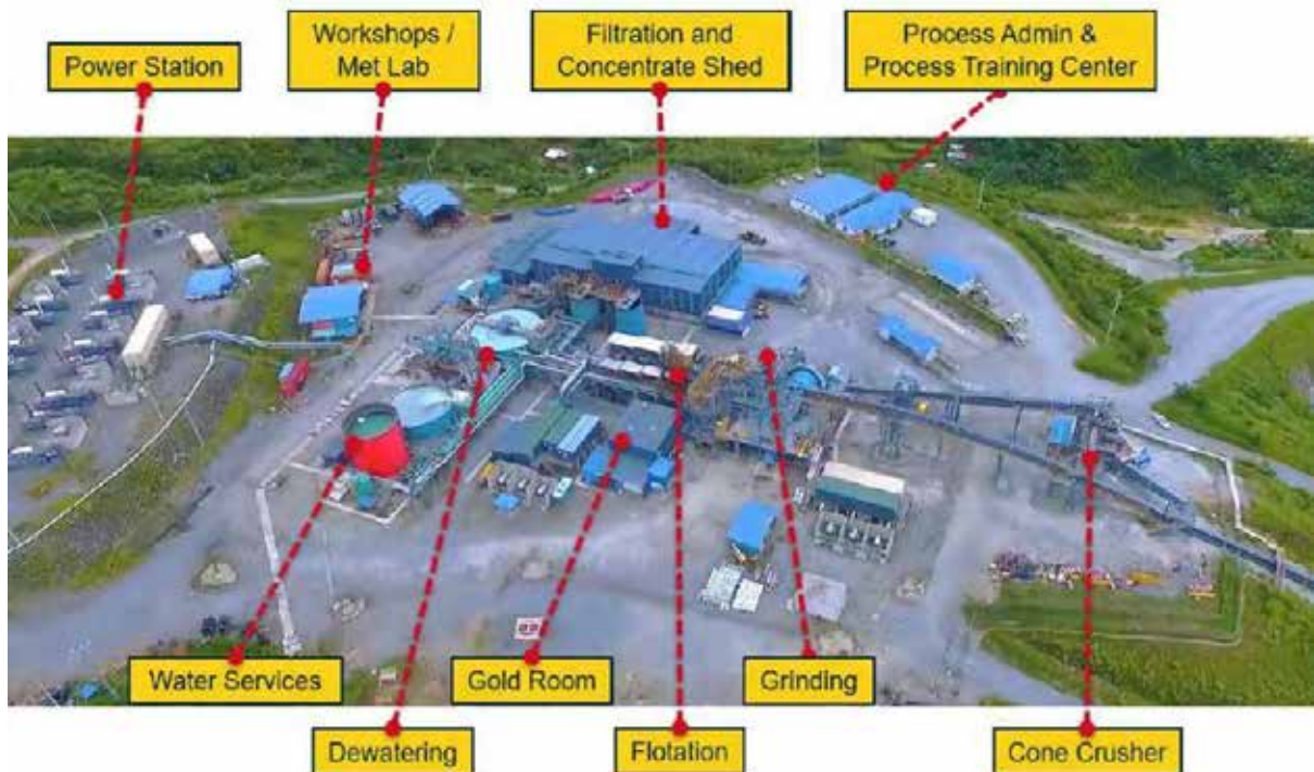
Figure 7-6. Process Plant Aerial Layout view
