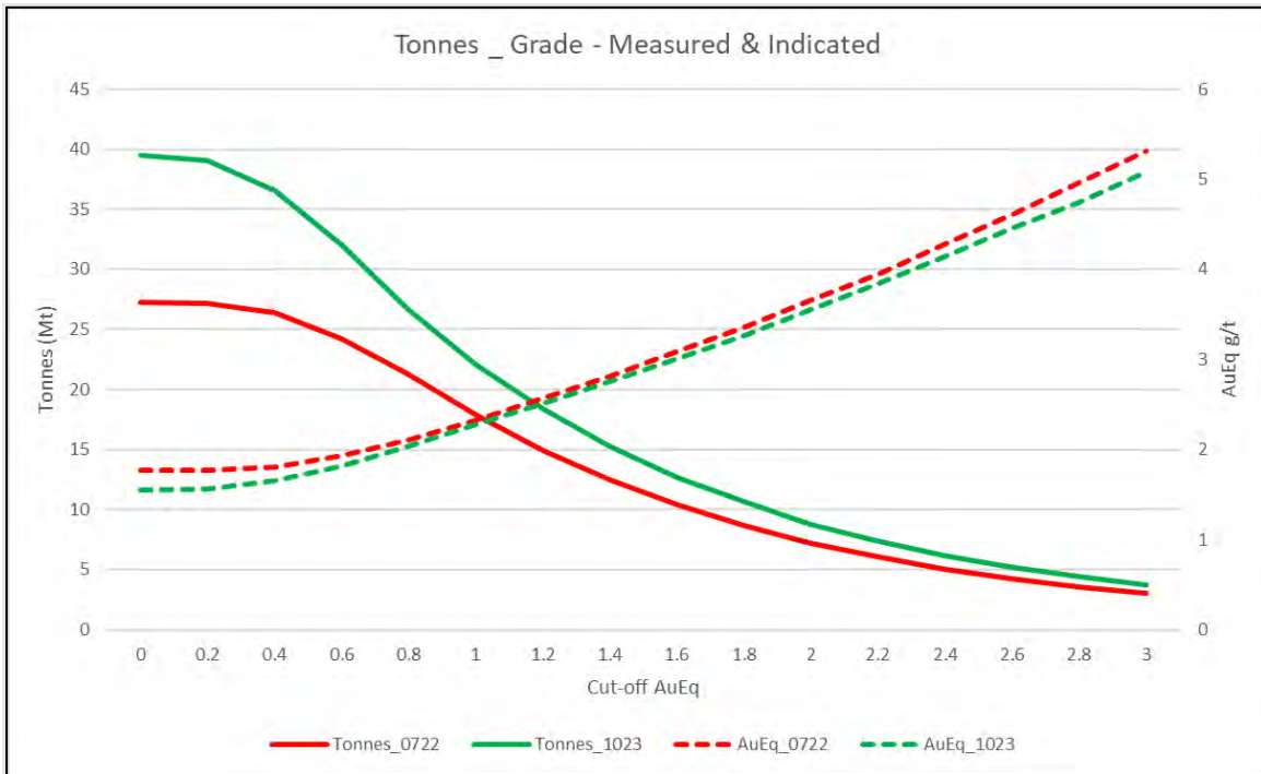
Figure 9-31. Grade Tonnage Curve Comparing depleted current 2023 vs July 2022 models (Measured and Indicated within Mineral Resource reporting solid)
