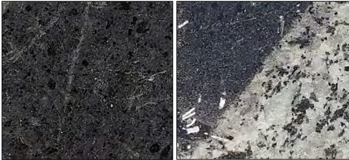
Photo 6-1: Dark Diorite (left) and Dark Diorite with sharp contact with Monzonite
