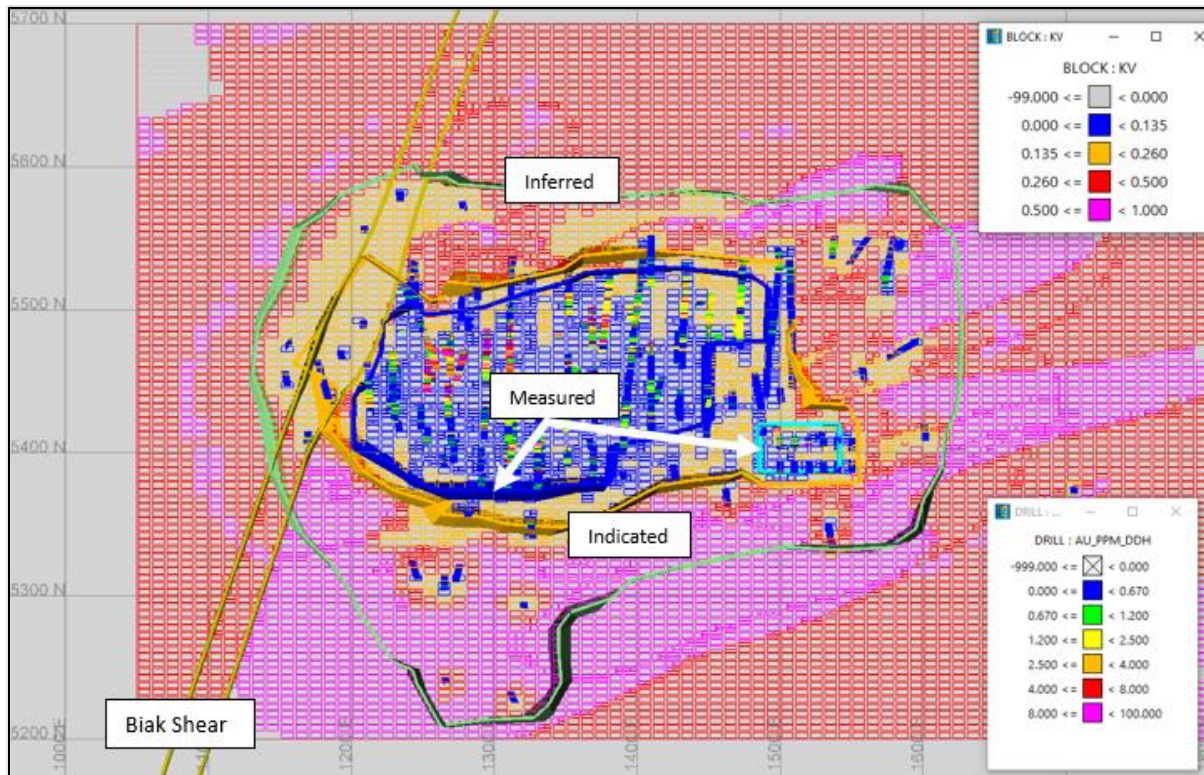
Figure 10-22: Block model (2355mRL +/- 7.5m) colored by Au OK estimate (KV). The drill holes colored by Au g/t. (Measured, Indicated, and Inferred strings shown, note Light Blue box - Measured for EBX).
